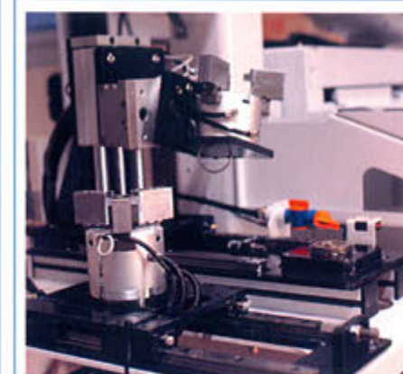
- Linear Scale (X and Z axis) - This option promotes high resolution and the highest machining accuracy.
